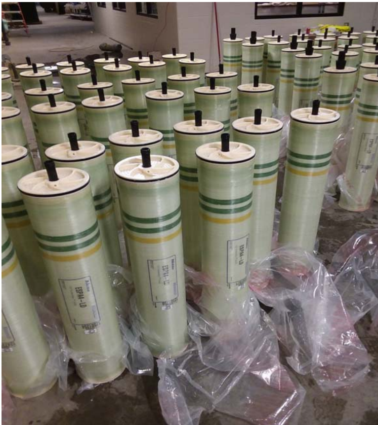
Hydranautics ESPA4-LD (low differential) Reverse Osmosis (RO) membranes elements being unpackaged and prepped for installation.
